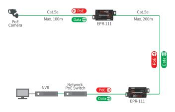
► Transmission distance may vary depending on the type and quality of cable, camera and environmental condition
